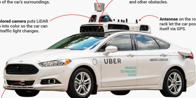
LiDAR modules on the front, rear, and sides help detect obstacles in blind spots.
